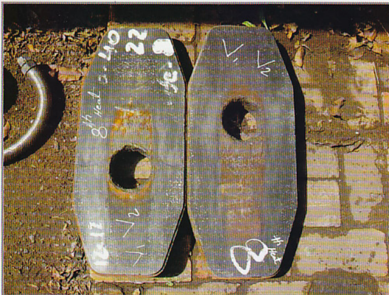
FF USED PLATE AFTER 8 HEATS, 170 TON LADLE - SLAB CASTER
